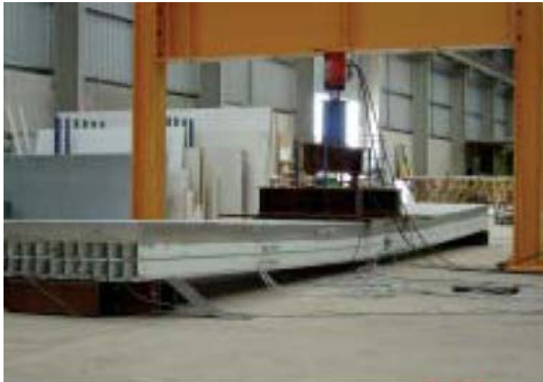
Figure 11.2c - 2/3 scale bridge deck load testing
