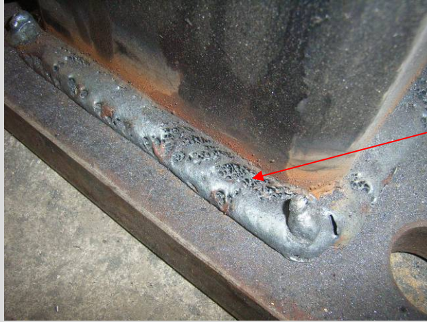
Figure 8.5.6(d) – View of the porosity in the weld
