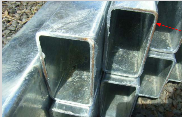
Figure 11.3.2(b) – View of incorrect dressing
