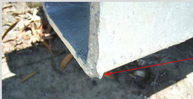
Figure 11.3.2(a) – View of the galvanising lump
