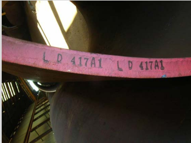
Figure 7.1.1(b) – View of the identification number on the edge of a steel plate
