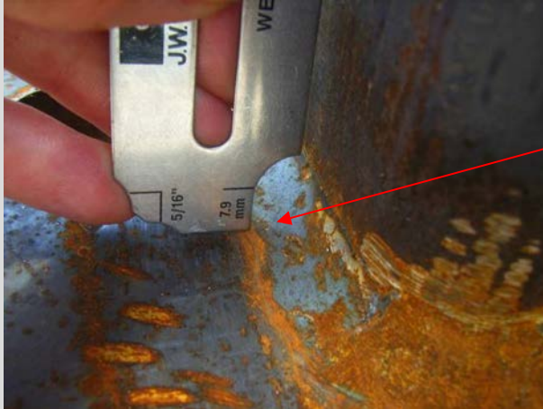
Figure 8.5.6(b) – Fillet weld throat thickness
