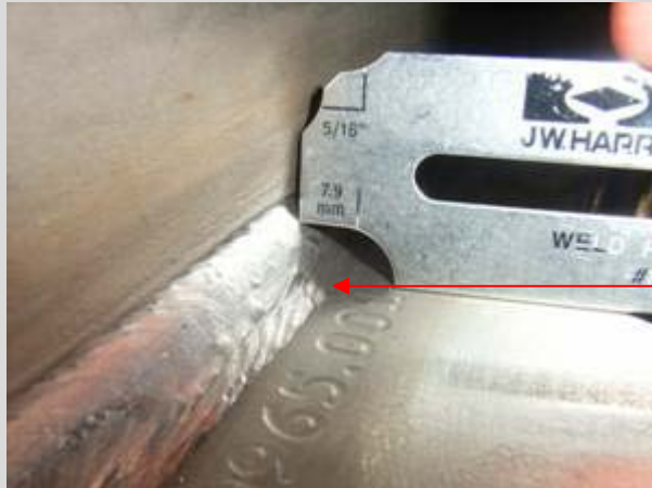
Figure 8.7.6(a) – Fillet weld leg length
