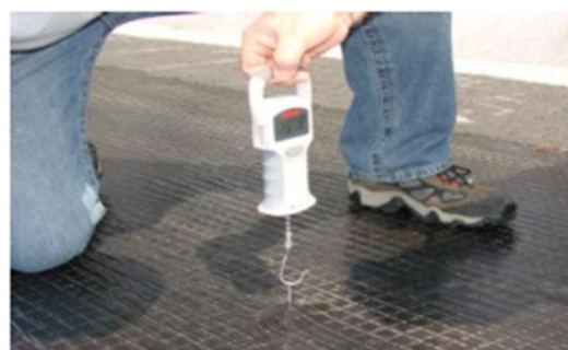
Figure 10.2.5 – Spring balance test to measure the construction bond strength
