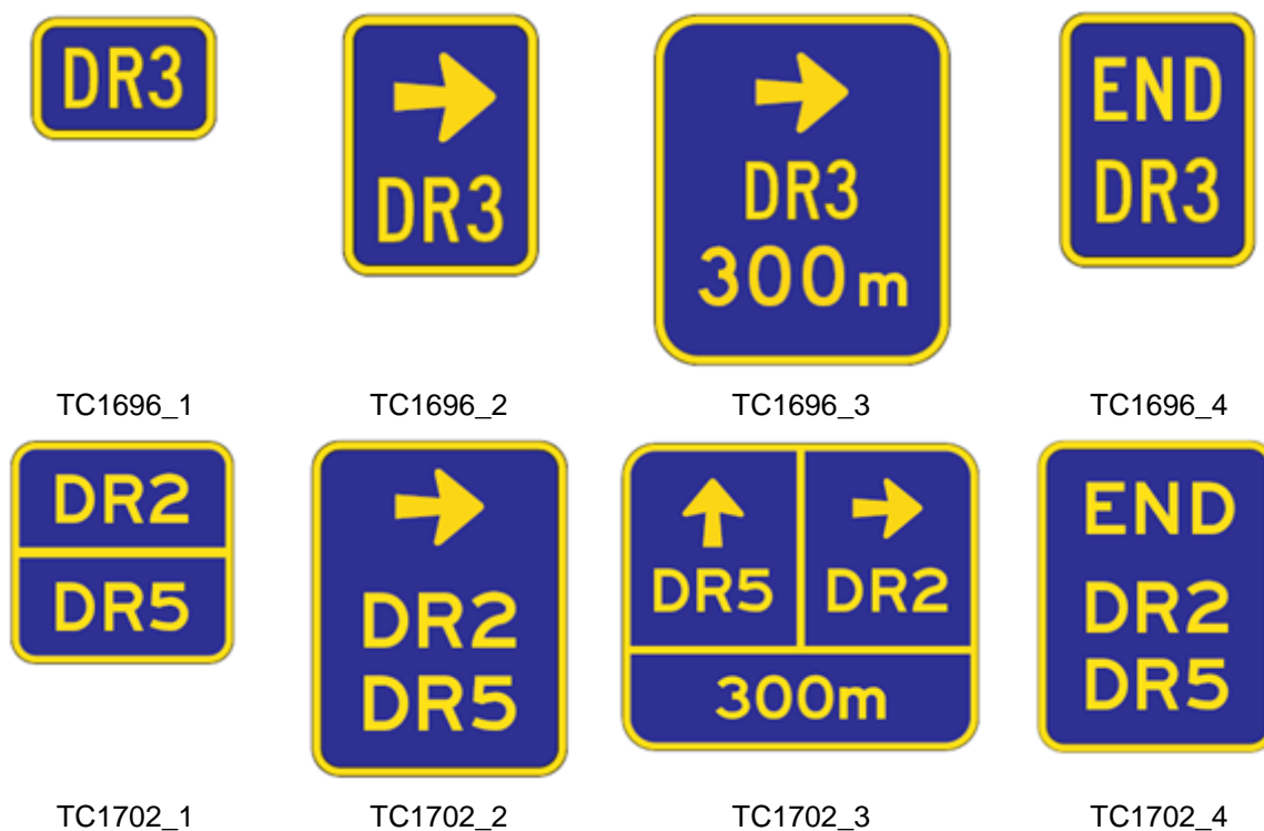
Figure 3 – Numbered diversion route signs
