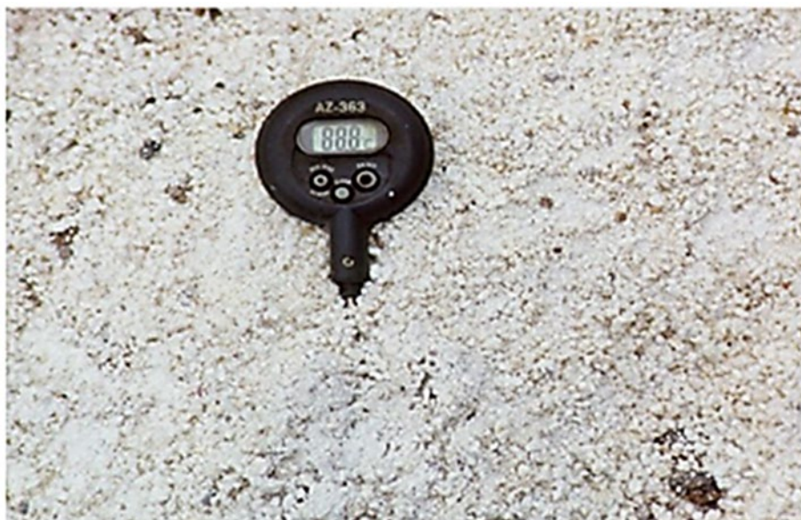
Figure 8.6.7 – Checking completion of slaking with temperature probe
