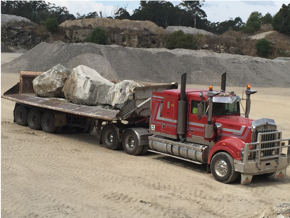
Figure 4 - Side Tipper with 5t to 8t Armour Rock
