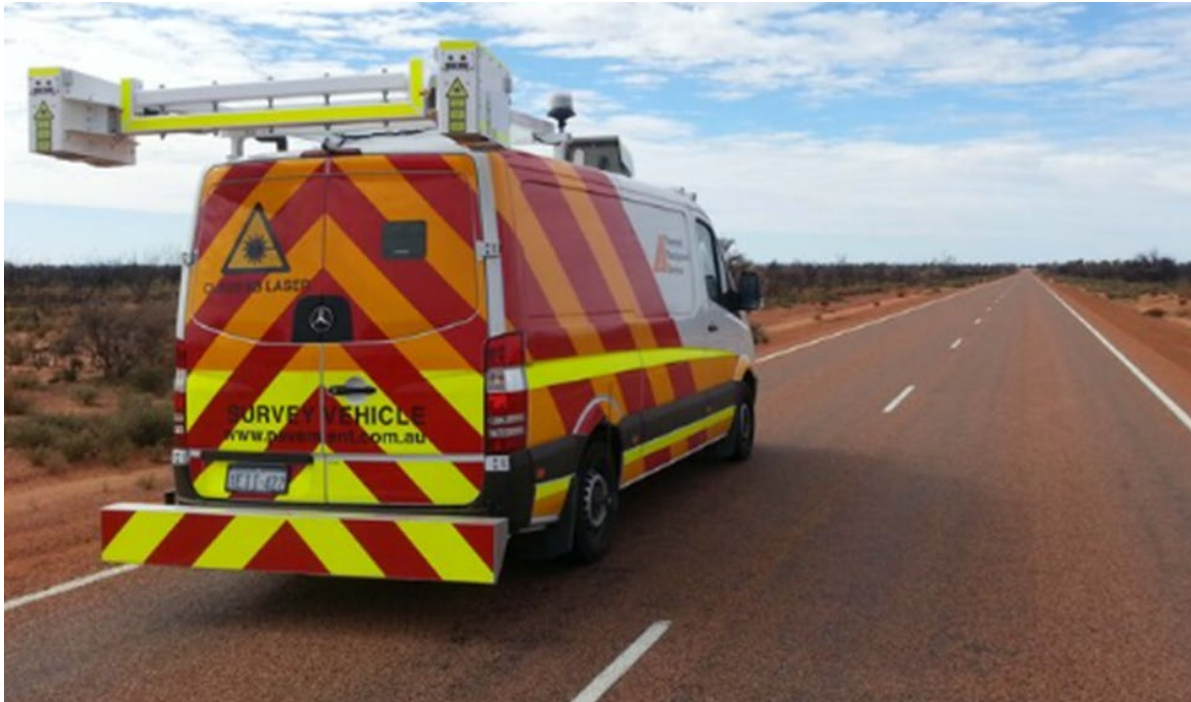
Figure 4.3.3(a) – Example of automated pavement condition and cracking survey equipment
