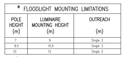
igstar Floodlight to be placed as near as is practical to the end of the outreach
