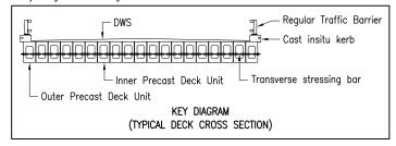
Skew angle is the angle between transverse stressing and the line perpendicular to the bridge centre line. Bridges with a skew angle ranging from 0° to 30° may utilise standard deck units with transverse stressing. Bridges with a skew angle ranging from 30° to 45° may utilise transverse stressing with shear keys or a reinforced concrete cast insitu deck slab.
