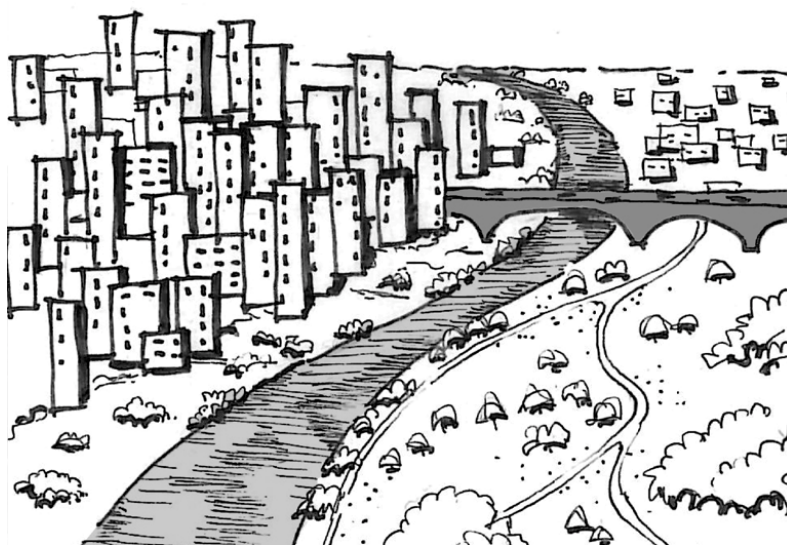
Figure A4-6: Improved legibility reinforced by clear edges that define different spaces and functions
