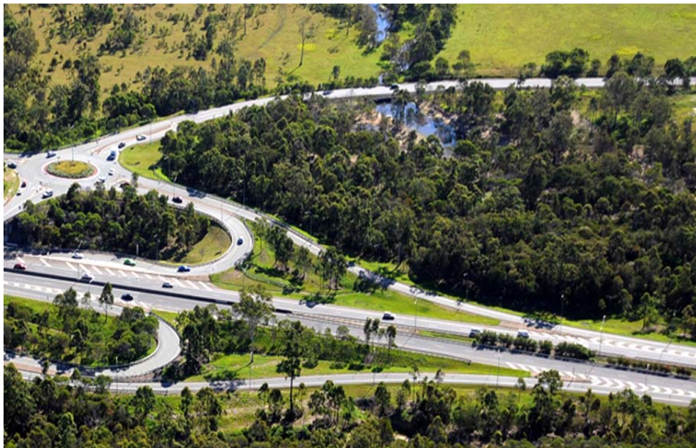
Figure C6-20: Effective rehabilitation of disturbed soils and water systems with landscape and revegetation treatments
