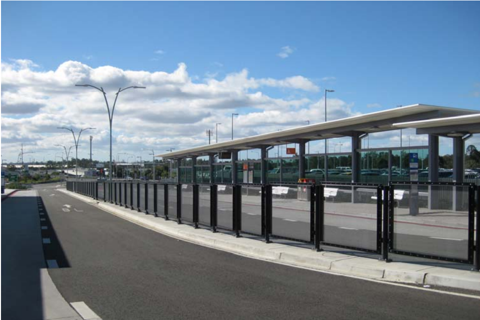
Figure C5-2: Improved surveillance through open style fencing
