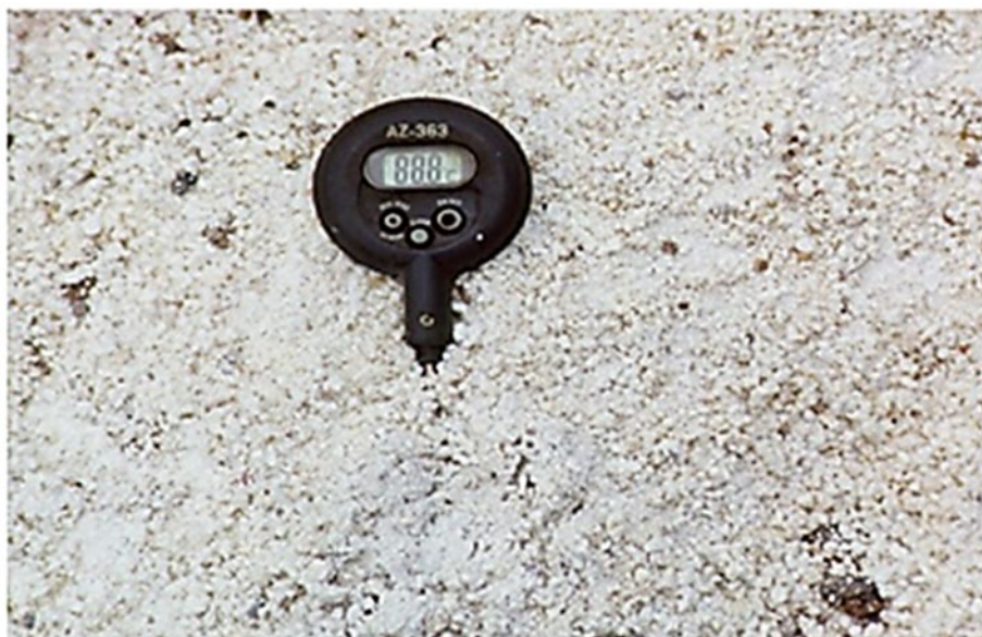
Figure 8.6.6.3.3 – Checking completion of slaking with temperature probe
