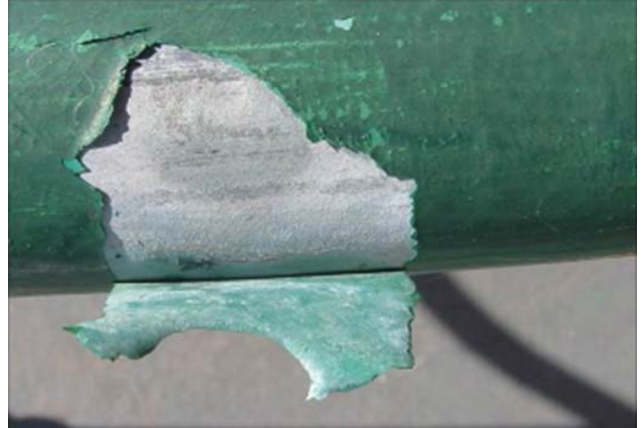
Figure 2.3.2b – Failure of paint system over galvanising
