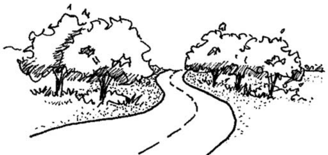
Figure C6-16: Roadway curvature responding to existing vegetation features
