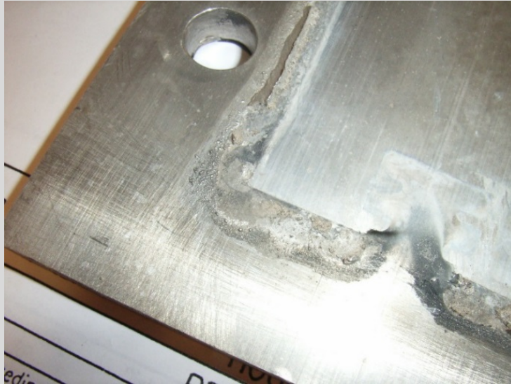
Figure 10.5.5.2(d) – Welding defect (lack of fusion)
