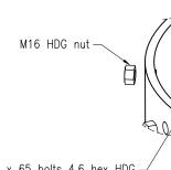
M16 x 65 bolts 4.6 hex HDG 52mm shank 13mm thread (supplied fasteners 12 sets).
