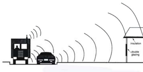
Control at reception point
