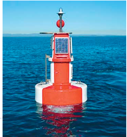
UV stabilised polyethylene buoy trial at the Fairway location at Gladstone
