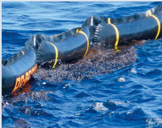
Oil booms were deployed as a physical barrier to trap and contain fuel oil spilled from the Shen Neng 1 when it grounded on Douglas Shoal
