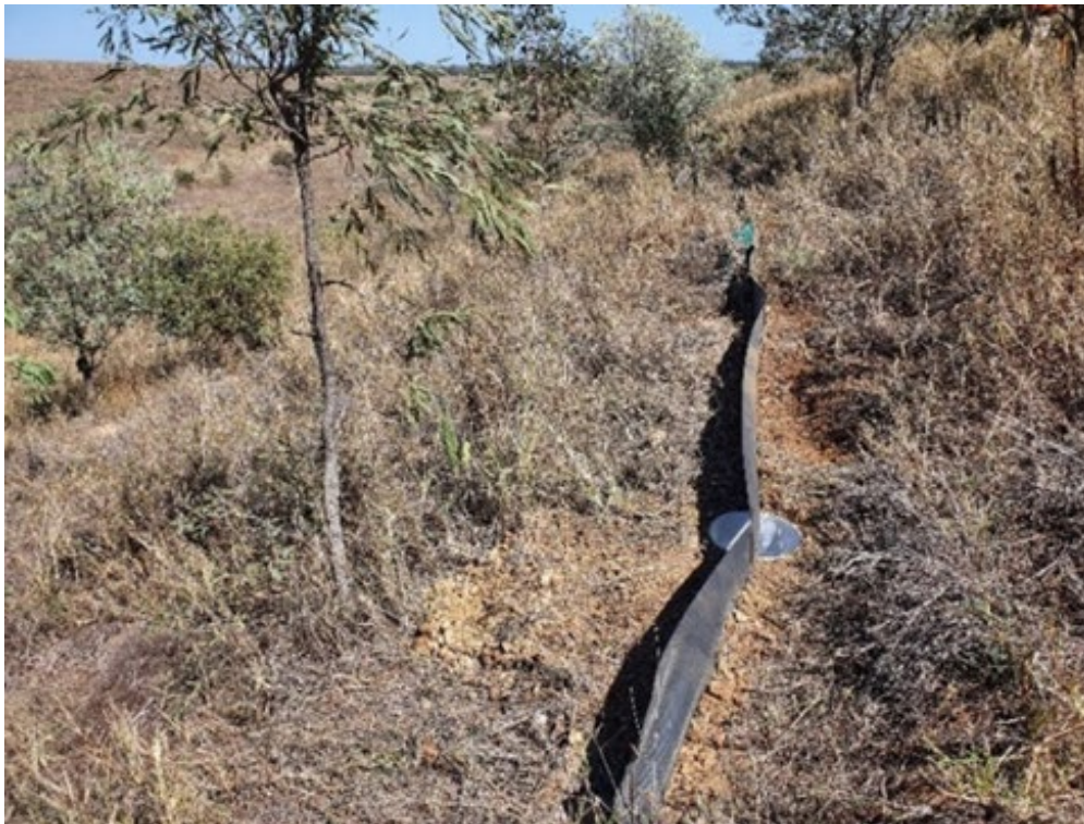
Figure A3(d) – Pitfall trap along a drift fence
