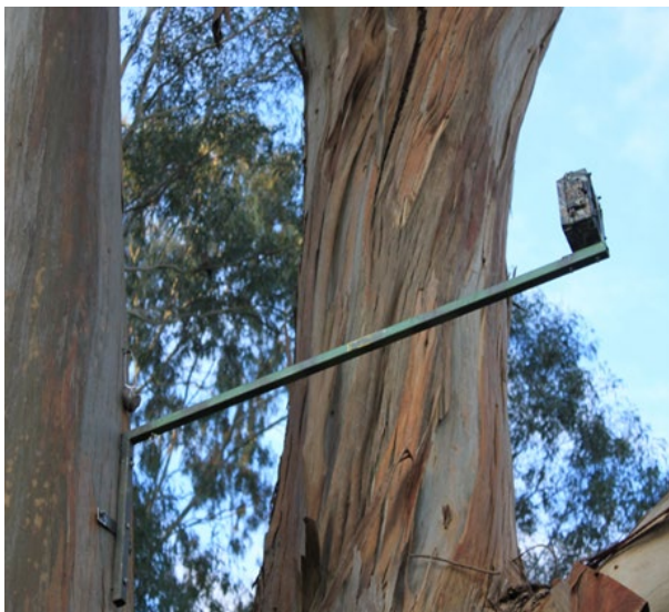
Figure A2(c) – Camera mounted on a bracket in a tree to survey for arboreal species
