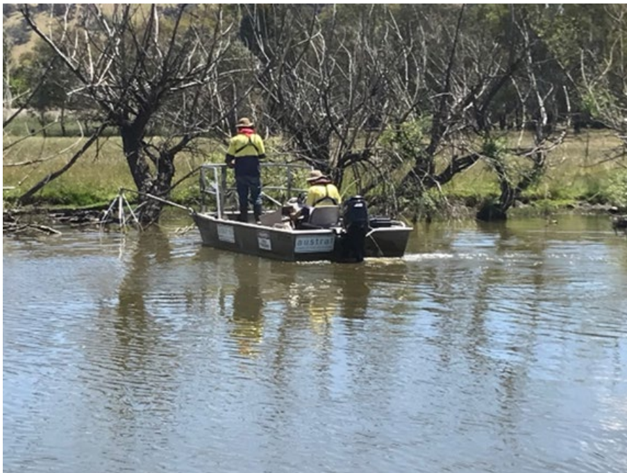
Figure A3(k) – Electrofishing undertaken from a boat
