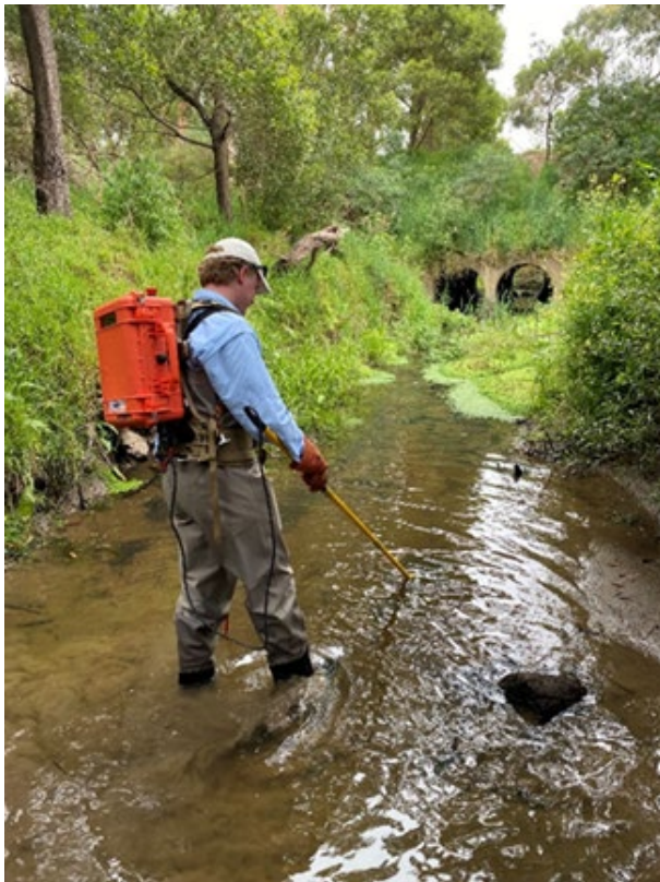
Figure A3(j) – Electrofishing using a portable backpack
