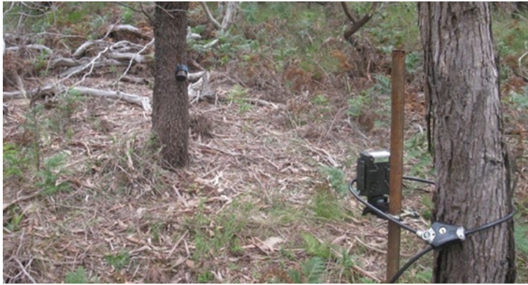
Figure A2(a) – Camera trap set up with bait holder
