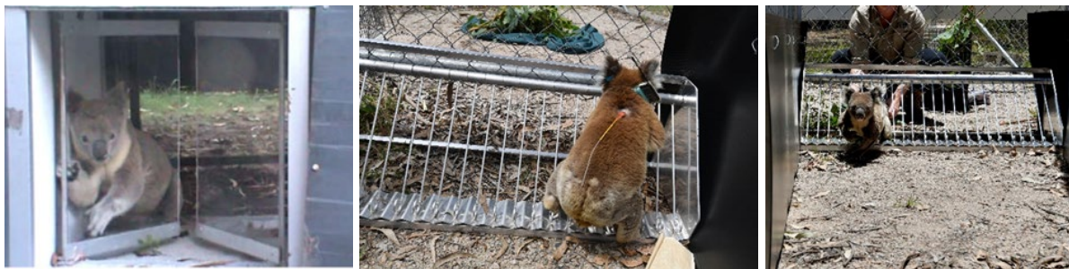
Figure 6.2.2.2 – Koala one-way gates being tested by Endeavour Veterinary Ecology
