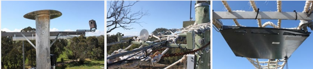
Figure 4.6 – Survey techniques installed on glider poles and canopy bridges (left) a passive infra-red camera; (middle) an active infra-red camera and (right) a PIT scanner.
