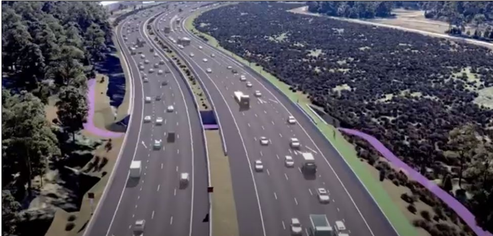
Figure 7(d) – Stylised graphic of the proposed fauna crossing underpass (indicated in purple)
