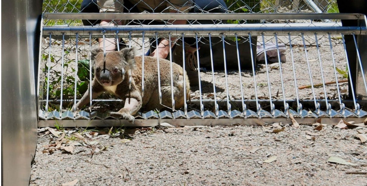
Figure 15.3 – Trial of rake gate for koala fencing
