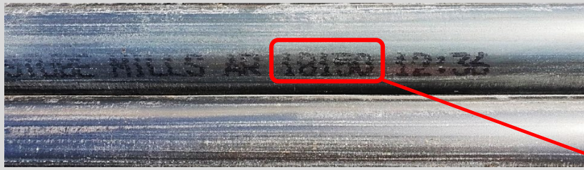
Figure 9.1.4(a) – Heat number on CHS
