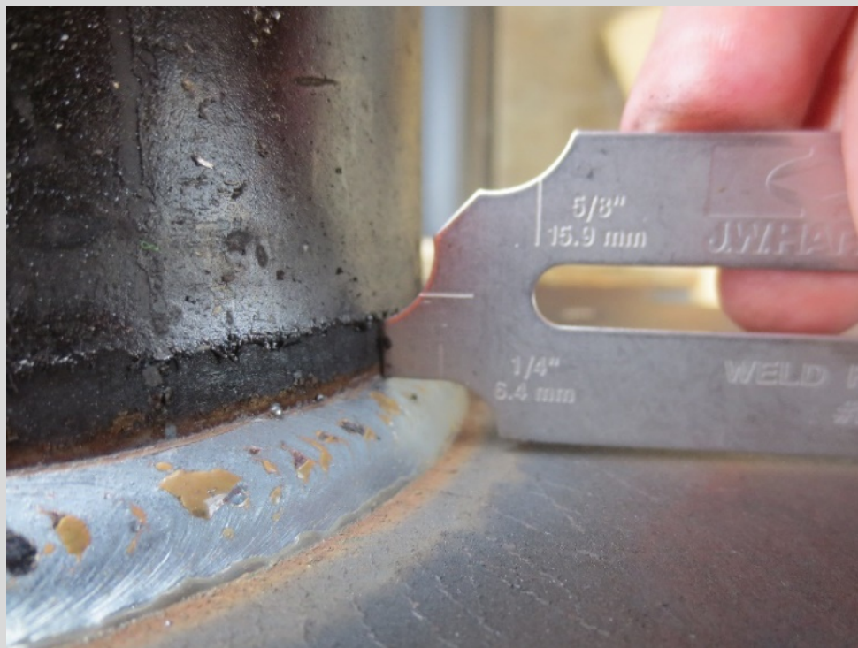
Figure 10.4.7.2(a) – Fillet weld leg length
