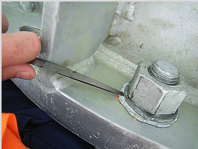
Figure 12.4(b) – Method of confirming correct torque applied
