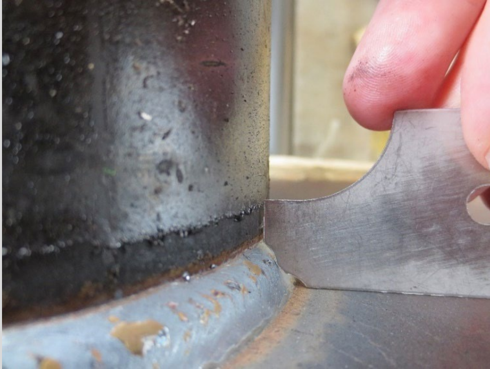
Figure 10.4.7.2(b) – Fillet weld throat thickness
