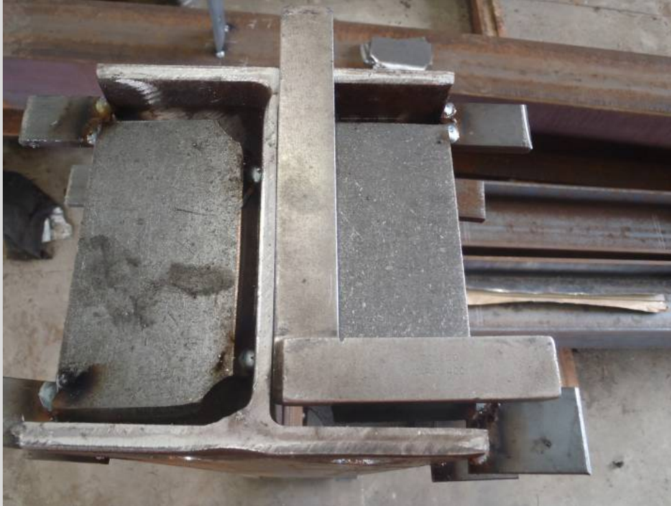
Figure 10.2.2 – Distortion of an I beam due to cropping
