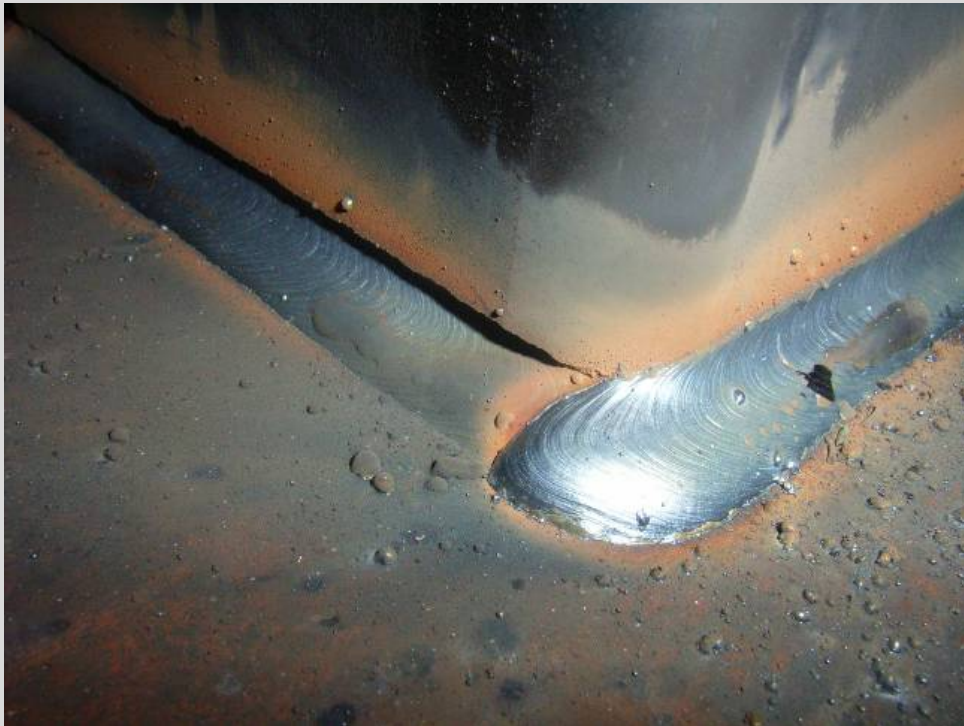
Figure 10.4.7.2(e) – Undercut in parent material
