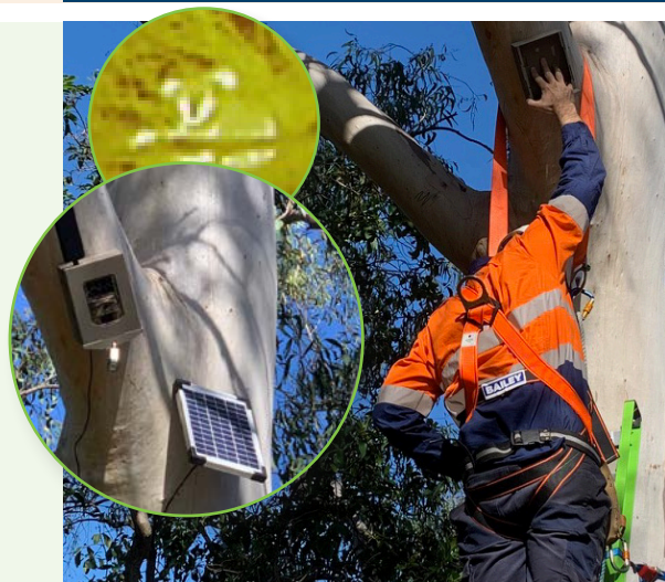
Right: TMR installing fauna monitoring equipment. Top left: Koala drone survey infra-red imaging. Bottom left: Monitoring equipment. Sources: TMR
