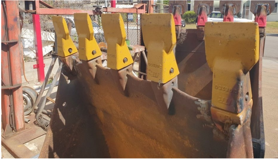
Figure 10.4(b) – Prefabricated excavator bucket's sharp or flare teeth
