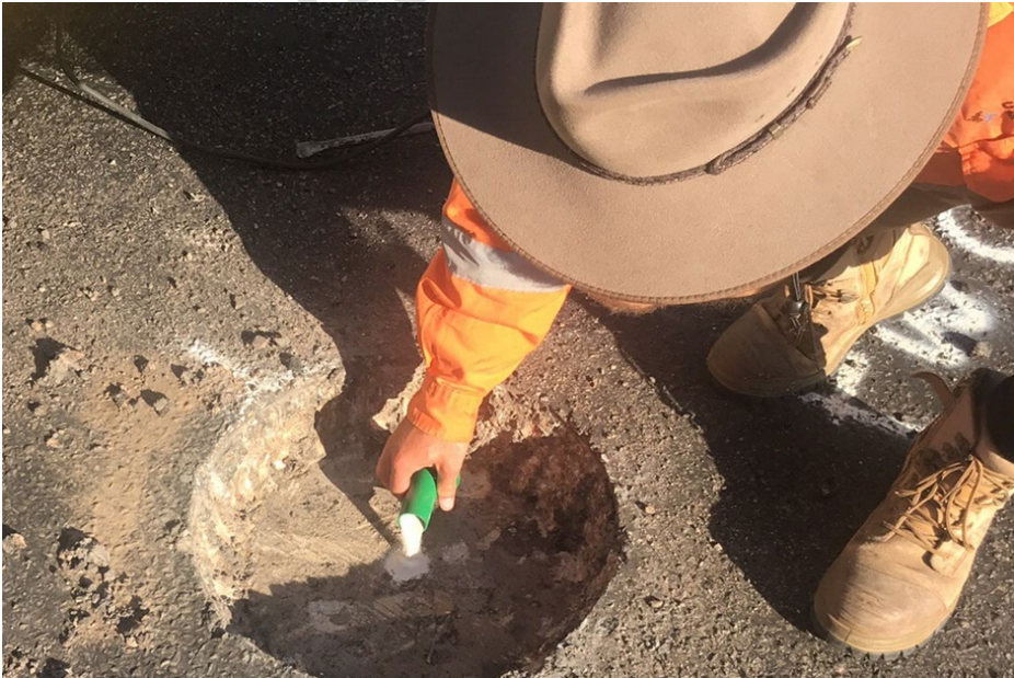
Figure A4 – Assessment of concrete bridge deck surface texture using sand patch test method
