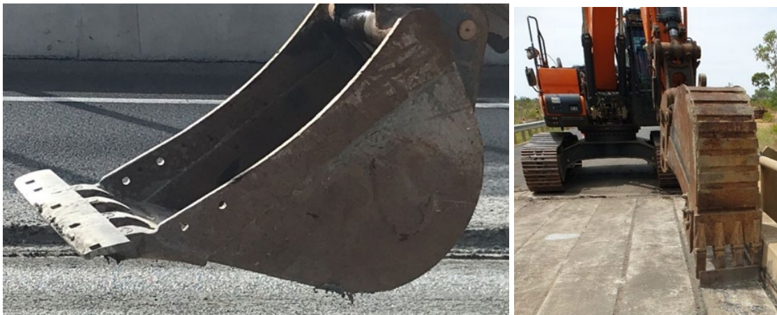
Figure 10.4(d) – Narrow trenching bucket with welded plate across the teeth
