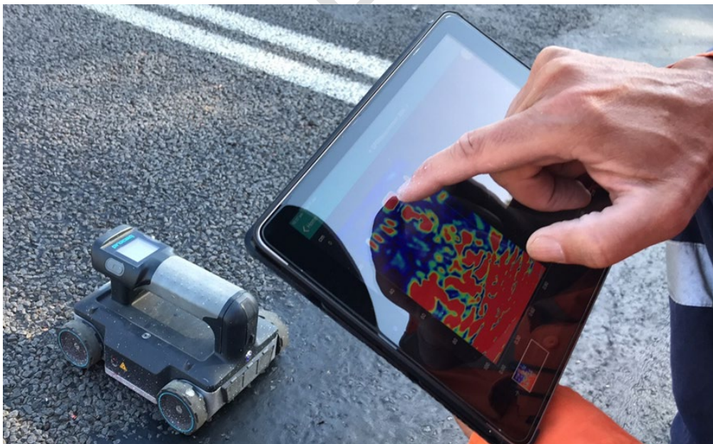
Figure A1 – DWS GPR depth scanning
