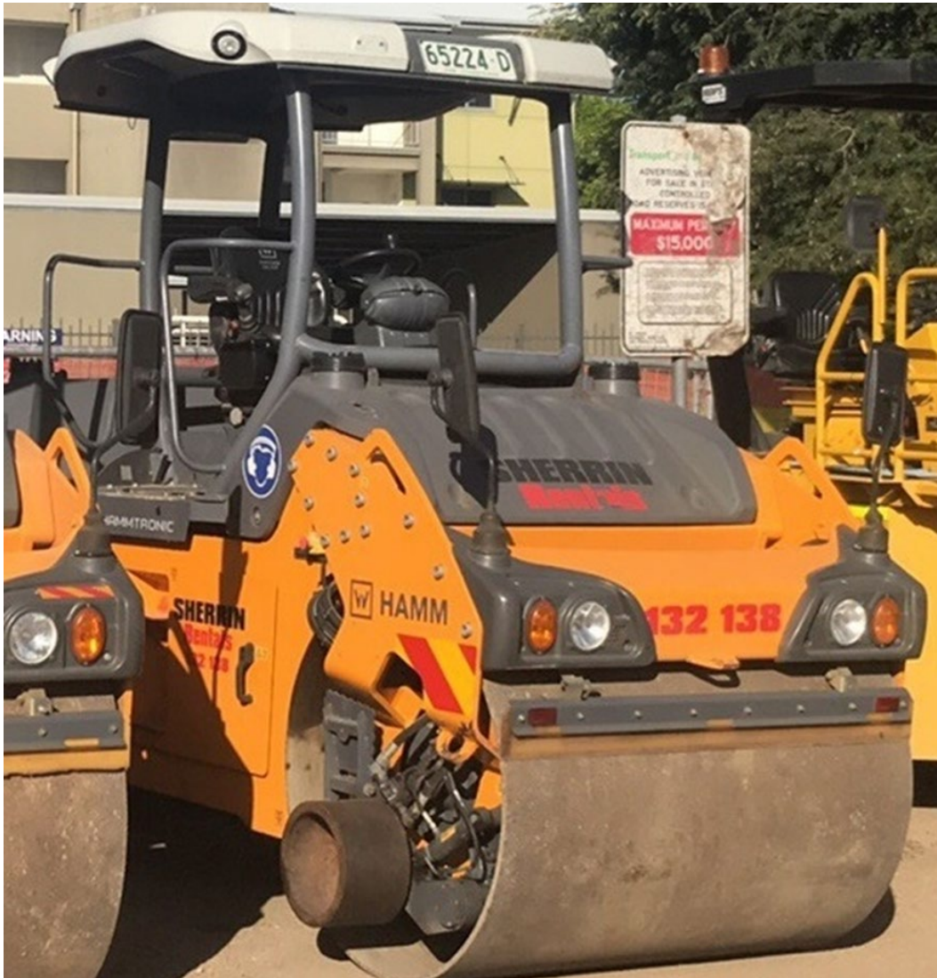
Figure 6.6(d) – Twin steel drum roller with a steel cylinder attachment to help compact the asphalt DWS edges at the concrete kerb
