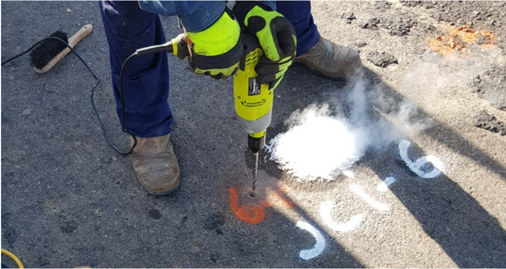
Figure A2 –DWS depth probing with handheld drill
