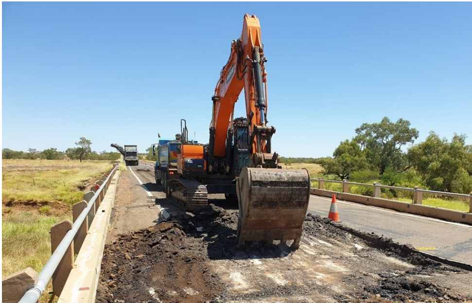
Figure 10.4(d) – Narrow trenching bucket with welded plate across the teeth
