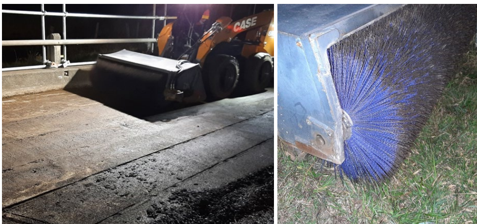
Figure 10.6.1(a) – A bobcat rotary broom with a combo sweeper brush attachment
