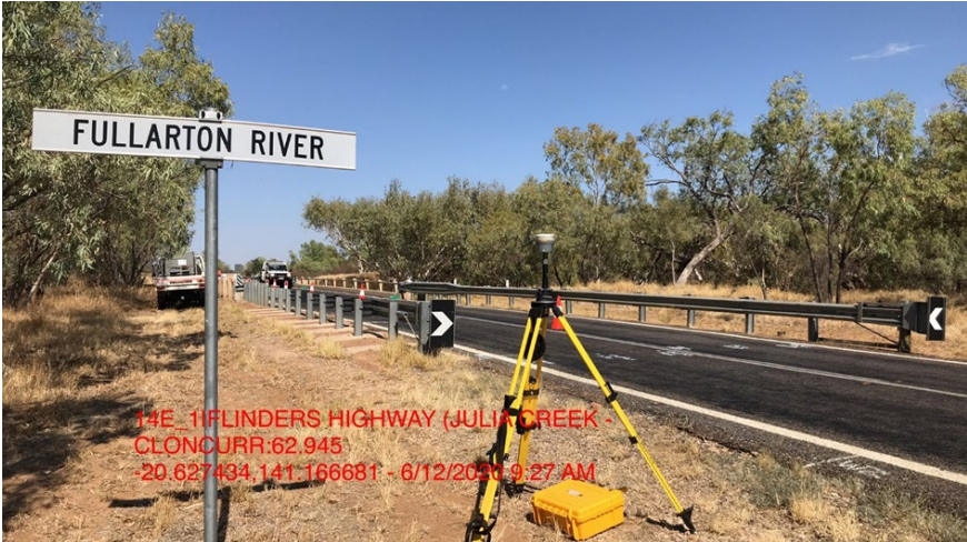
Figure A5 – Survey pick up of DWS scan and locations, DWS crossfall, and gradient
