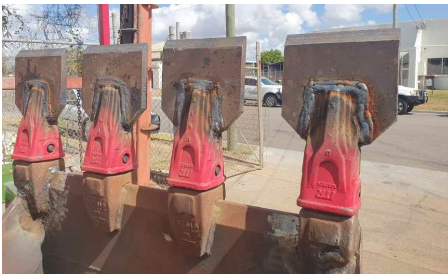
Figure 10.4(a) – Custom made excavator bucket's sharp or flare teeth
