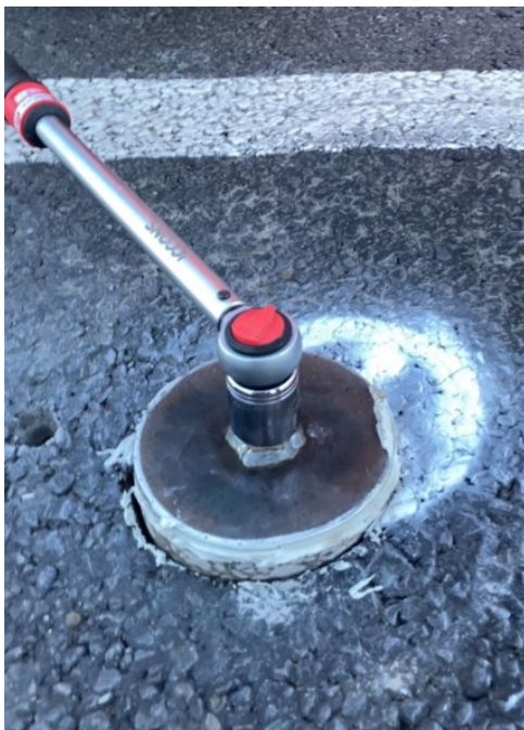
Figure 10.2(b) – A torque wrench used to spin the plate apparatus to assess the bonding
