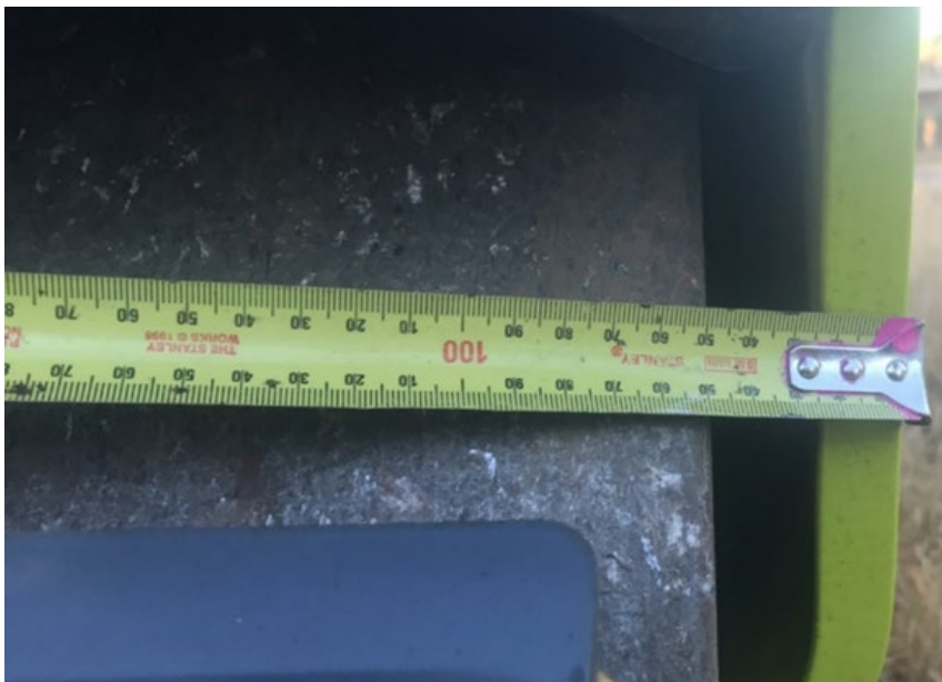
Figure 6.6(c) – Twin steel drum asphalt roller with approximately 60 mm offset to the drum on each side
