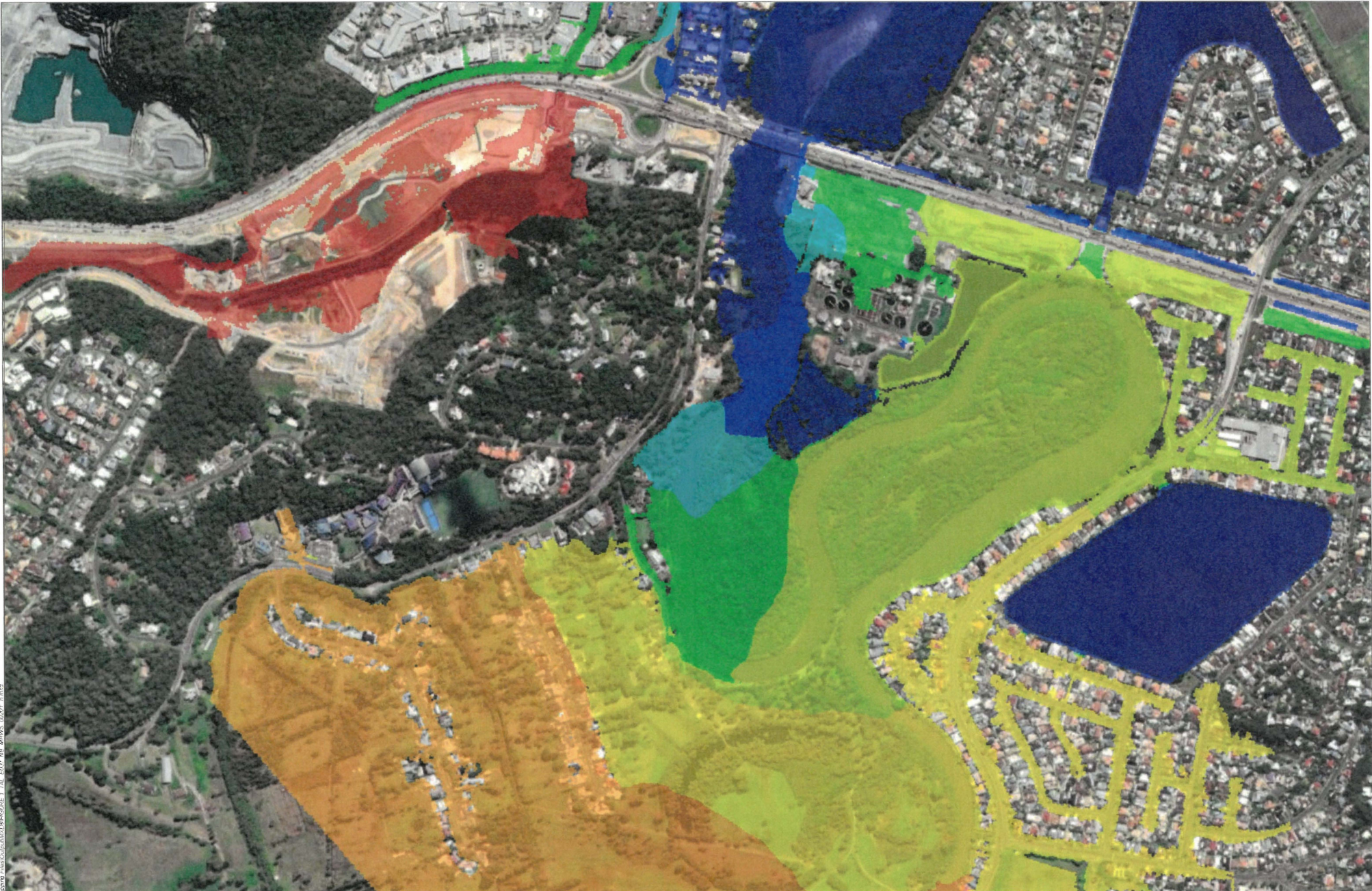
M1 B2PB - Tallebudgera Creek Construction Flood Impact Assessment Pre-Construction Conditions (E037) Peak Flood Levels - 5% AEP
