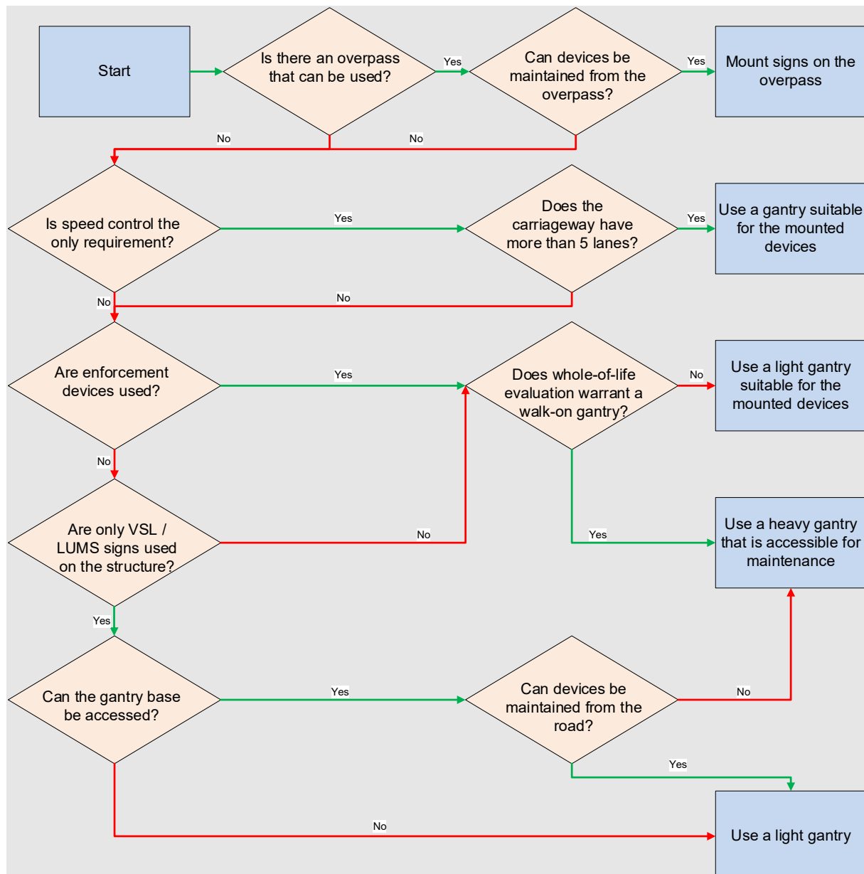
Figure 12.4.6 – Determination of Gantry Type for ITS Devices
