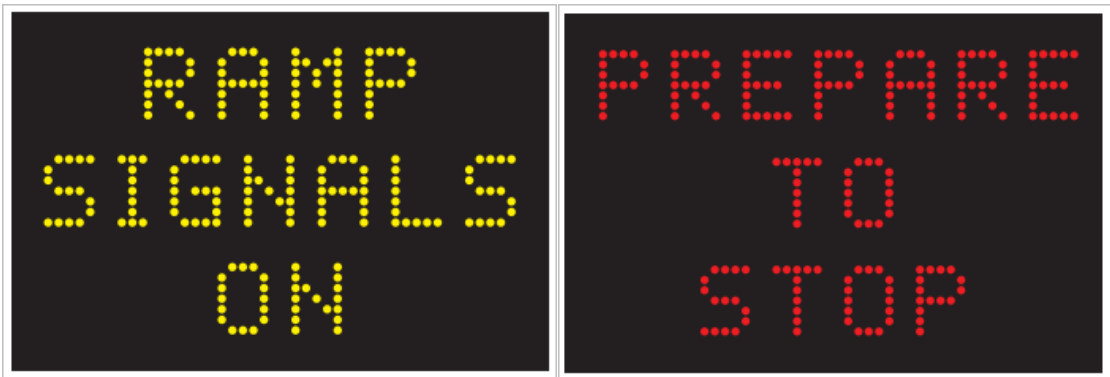
Figure 11.5.7 – Ramp signal warning signs TC2290_1 and TC2290_2.
