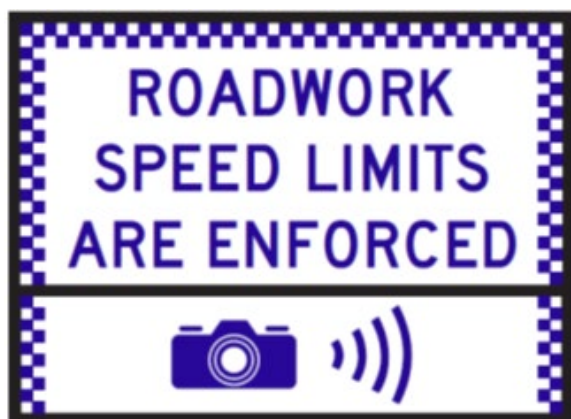
Figure 5.5.4(a) – Multi-message sign arrangement for planned camera enforcement (undertaken outside the requirements of Technical Specification MRTS02 Provision for Traffic)
