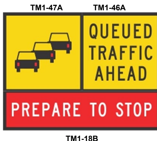
Figure 4.8 – Queued traffic ahead multi-message sign assembly
