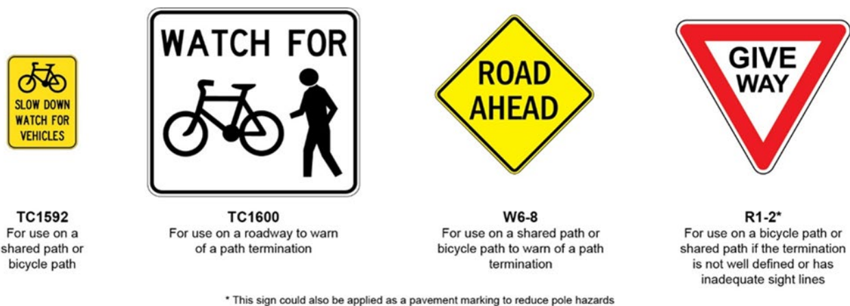
Figure C.9 – Signs used for slowing people riding bikes and warning of a path termination
